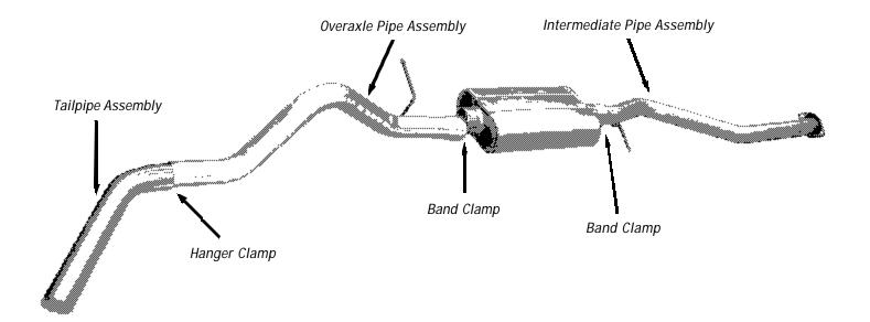
WARNING: Support your vehicle with proper jackstands or ramps rated for the total vehicle weight. Place stands so that the rear axle is allowed to hang free for easy system removal.
